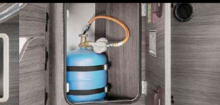
13 Gas cylinder compartment (Campingaz R 907 2.75 kg)
