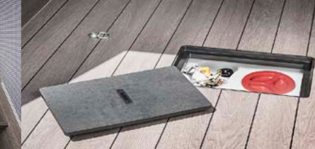
5 Fresh water tank cleaning hatch
